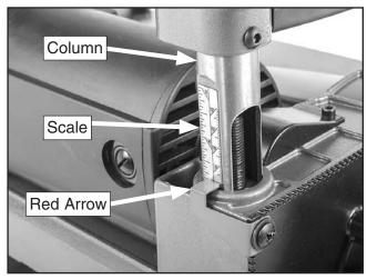
Figure 15. Positioning elevation scale.
